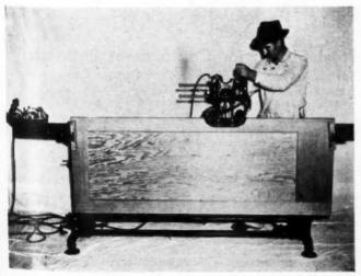
ABOVE at top: Contractor Zern's door fitting machine showing use of electric router. Lower view: Power mortiser in use; note electric planer at left end of machine, placed for immediate use. KNAPP ACCESS PANELS Simple and Easy Ito Install .....
