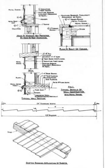
FIG. 2. 4. WEATHERBOARD SIDING.
