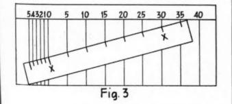
Below is the finished strip, or paper scale, which can be used to obtain the measurements of all plans and elevations of the same set of drawings.
