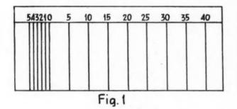
Second, I take a strip of drawing paper about one-half inch wide and five inches long. This is placed upon the magazine drawing to be copied, along one of the longer dimensions of an exact number of feet, and two marks representing this distance are marked on its edge. (As a sample, 30 is being used.)
