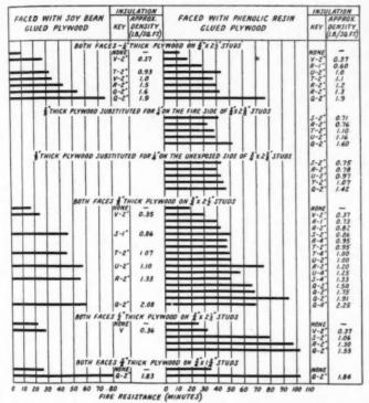
FIGURE 2.—Fire resistance of plywood wall sections filled with various amounts of mineral wool batt insulation.
