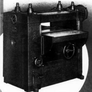
One-piece main frame of great sturdiness totally encloses and transmission, giving operator complete safety. One-piece so section provides great rigidity and vibrationless operation. Infinitely variable range of feeds, with safety foot said quick release.
