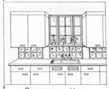
HOUSEWIVES like plenty of daylight on their kitchen work counters and frequently upper cabinets make this difficult. By taking out sections of the walls where bearing is not essential, glass block can be inserted as shown at the left. Construction details appear below.
