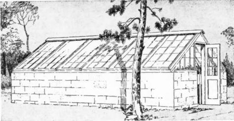
THIS greenhouse will be useful for starting transplanting stock on a farm; block sidewalls reduce the amount of lumber required.
