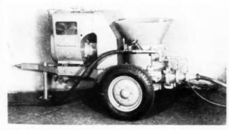
Chassis mounted concrete gun shoots various materials into place.
