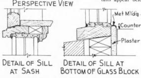
JOINTS at top and bottom of block are caulked.
