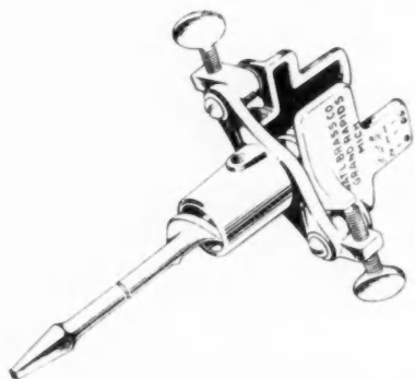
Learn about the Dexter Bit-Guide — the tool that gives streamlined, factory production method to Dexter-Tubular installation. Simply clamp the Bit-Guide on the door — self-centering, no measuring — guides the boring straight and true. Ask your dealer for a demonstration and complete details.
