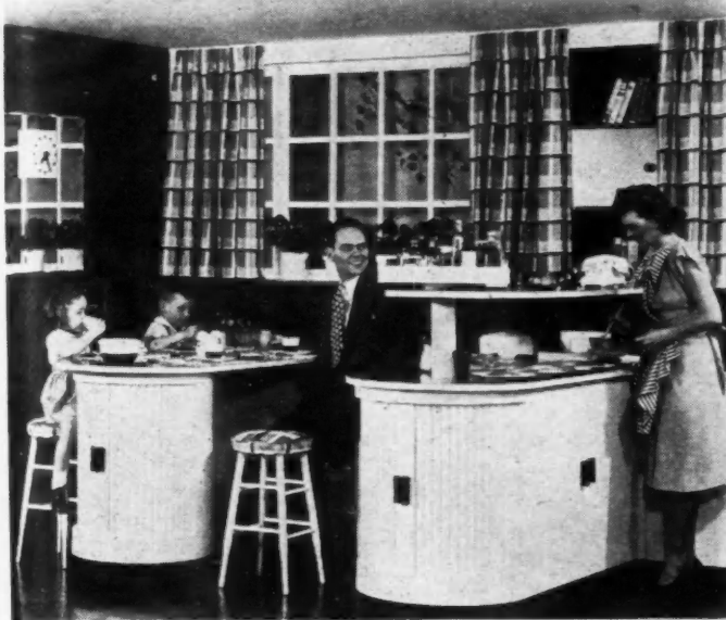
LEFT: In this kitchen a panel of beveled-edged mirror, on which a clock is mounted, reflects colorful interior. Novel curved-end work counter with roll-type sliding doors, upper shelf and matching, convenient breakfast bar have easy-to-clean Vitrolite glass surfaces.
