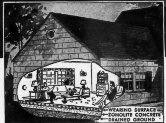
Cutaway view of basementless house showing how layer of Zonolite Insulating Concrete laid on the ground and covered with a topping of ordinary concrete eliminates loss of heat downward.
