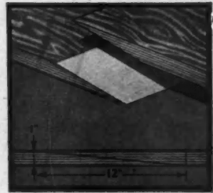
Scarf Joint, Ratio 1" to 12"
