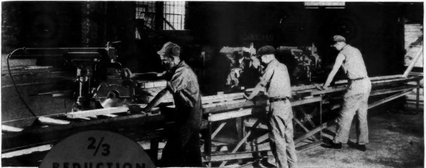
Three Walker-Turner 3 h.p. Radial Saws are set on channel beams on a 40 foot conveyor table which reaches to the railroad siding. The saws are set by control handles placed at both ends of the table.
