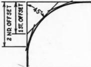
IN offering the following, Richard M. Barner, Colwyn, Pa., says: "Here is a method, I use to round off corners without the aid of a template. The method is both fast and accurate. Lay out radius full-size on board. Scribe first and second offsets as shown."
