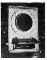
which is attached to the main plate by four bolts; and a clean-out door and check draft. The clean-out door is directly under the smoke pipe which makes it possible to clean the flue without disrupting the furnace pipe. It also eliminates the need of a check draft door in the furnace pipe; by attaching the draft regulator chain to the bottom of the clean-out door, the furnace can be checked and the flue cooled.
