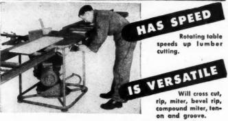
Here is a speedy, money saving saw adaptable to a wide variety of applications. It is portable - easily taken to the job, can be carried by two men. It will rip to a depth of 4 inches and cross cut a 3" x 12". Furnished INDUSTRIAL PLANTS with gasoline engine or electric motor drive. Write for Bulletin 132.
