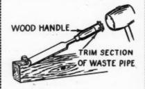
TO KEEP wooden handles from splitting when driven by hammering, use left over ends of plumbers nickel and chrome-plated trim as a band for the end. GEORGE T. MANN, Fort Meyers, Fla.
