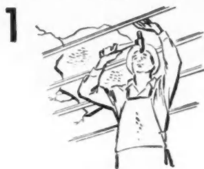
1 Nail furring on 16" centers, right over old plaster.
