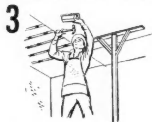
3 Clinch fasteners. See direction sheet for simple method.
