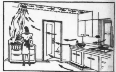
THE modern functional kitchen should have a ventilator directly over range
