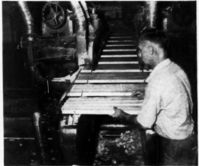
6 EVERY lug carries pay load of stiles through double end tenoner. Stock sash are being produced in big quantities
