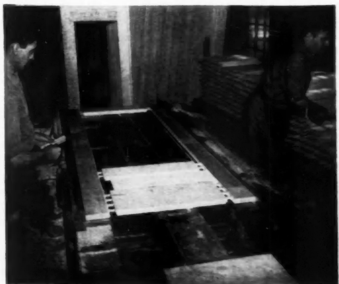
9 POWER CLAMP turning out a combination door. Operator on left is ready to insert an instruction sheet for builders
