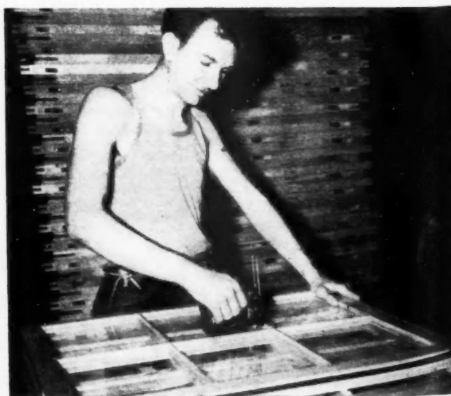
7 AUTOMATIC trigger-operated tinner drives diamond points to fill-in-and-tin glass into the sash before they are glazed
