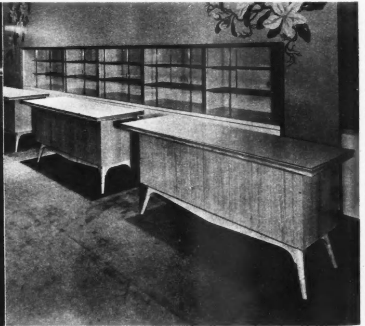
TAPERED hardwood spindles are combined with plywood to make these two types of display furniture for a Buffalo department store
