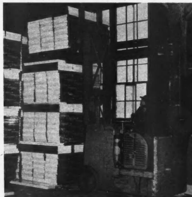
7 THIS particular truck has a total lift of 108 inches, permitting piles 9-feet high to the bottom of the top unit. Easy piling of high stacks in warehouse is demonstrated here
