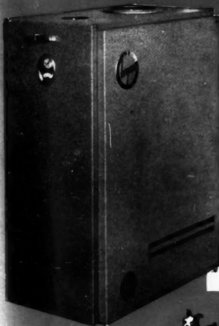
MODEL 26 —A. G. A. ratings sq. ft.: Steam 230-600, Water 360-1920. Inputs: 67,500 to 360,000 btu per hour. For moderate size hot water and steam radiation heating systems. Features maximum heating surface, with water tubes surrounding the combustion chamber. Jacket is asbestos-insulated, completely encloses boiler and controls... A favorite for home radiation heating systems.
