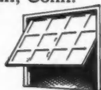
2. "SLIDE-UP" For old or new doors. A simple weight-box, sand-filled, balances the weight of the door.
