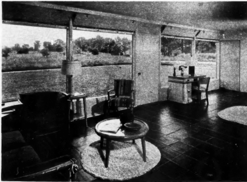
TILE blocks which are finished on top surface form panels for radiant heating system. No additional flooring or floor covering is required
