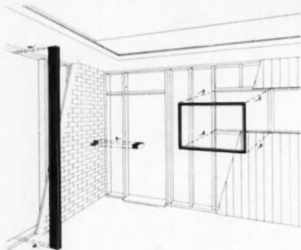
MATERIALS made in multiples of four inches reduce cutting and waste, and can be fitted together in a simple and orderly manner where building was planned for their use
