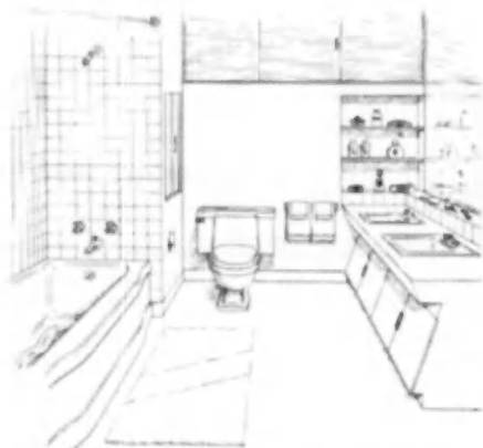
REVISED layout of bathroom contemplates a relocation of fixtures based on the use of high windows on the outside wall
