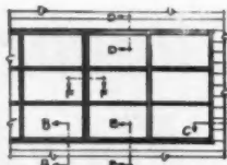
PARTIAL ELEVATION SHOWING SUGGESTED METHOD OF JOINING TWO OR MORE WINDOW WALL FRAMES.
