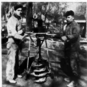
POWER POST HOLE AUGER operated by two men does the work quickly and neatly
