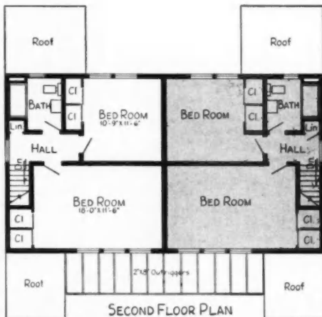
SECOND FLOOR PLAN. Each unit has two bedrooms and one bath
