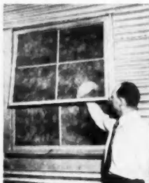
TRANSLUCENT qualities of flat plastic laminate is shown here with man's hand and handkerchief partially showing through the panel
