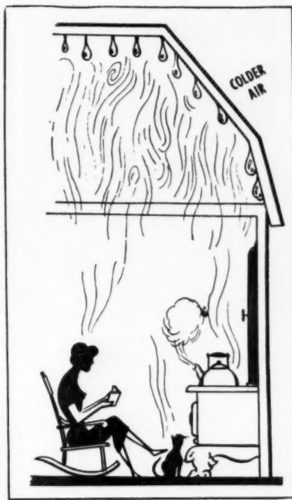
Condensation forms when the capacity of an air space at a given temperature is too small for the amount of vapor present.
