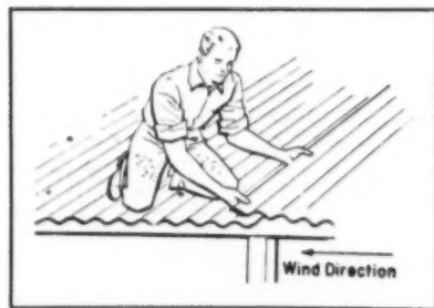
Lap sheets 1½ corrugations, open edge leeward. Use mastic seal under open edge
