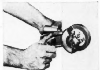
Clamp SPEEDRIL to door with Adjusting Screw, tighten with 'C' Clamp Screw.
