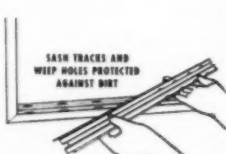
No more dirt or bug trash—for you or the owner. The sash track is protected with a removable zinc cover plate.
