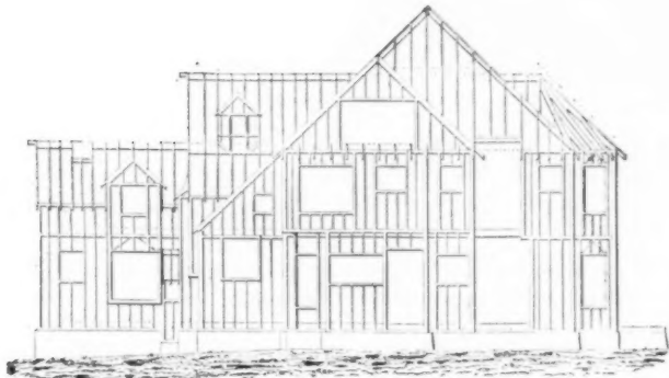
A Study in Suburban Architecture—Framing Plan, Showing the Timbering of Porch and North End, 1/4 Inch to the Foot
