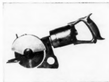
1924—The first Skilsaw, one of the pioneers of a whole new era of power tooling on the building site
