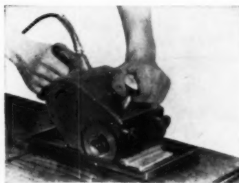
An early (1932) finishing sander made by Porter-Cable. It had a drum on which an abrasive sheet was mounted
