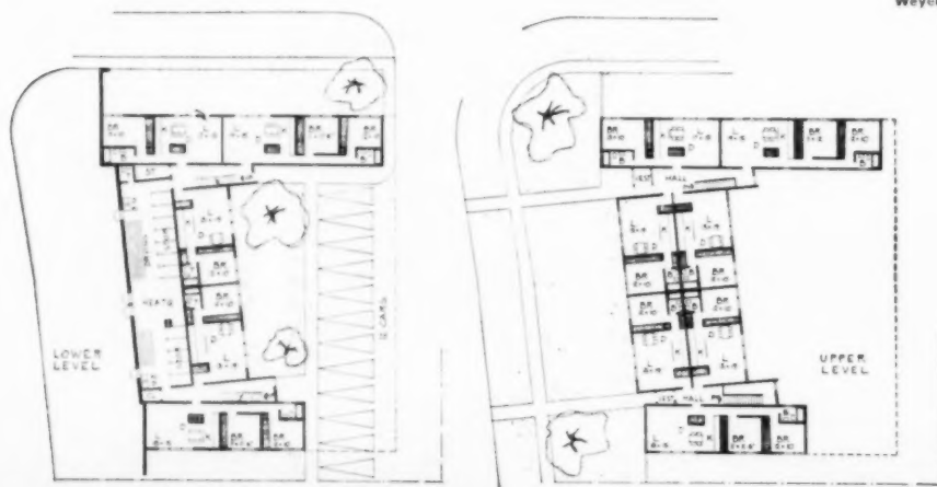
Four two-bedroom units are placed in wings. Utility room has private storage space for each tenant
