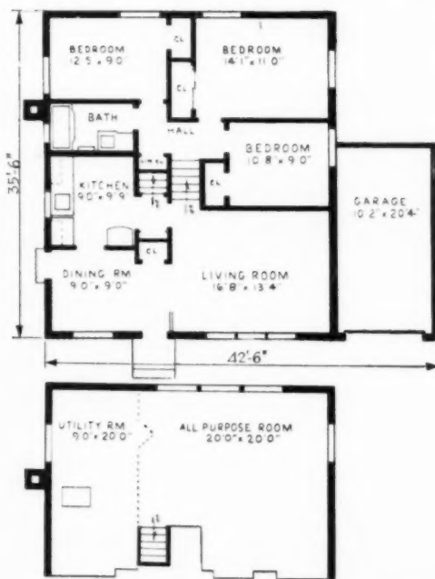
Broken line in lower level plan indicates how large multi-purpose room can be created
