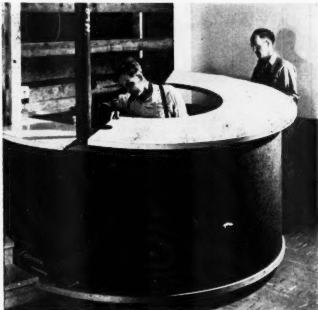
Formica was added to the top, and a 1x3-inch strip attached around the bottom
