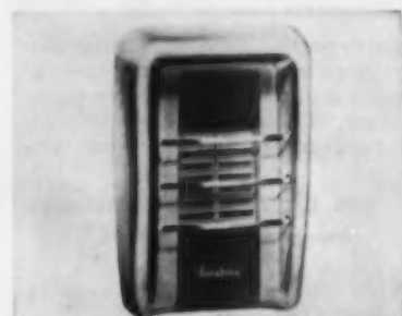
AB15223 — WALL HEATER — Armstrong Products Corp., Dept. AB, Huntington 12, W. Va. Made for any type gas and sized to fit standard openings, Model 108 is 21 in. high, 13 in. wide; recessed section is only 3½ in. deep. The front is one piece of white porcelain and panels are platinum gray, a popular bathroom shade. Lower panel is hinged to give easy access to the valve and air regulator. 8,000 Btu unit is unvented, AGA approved.
