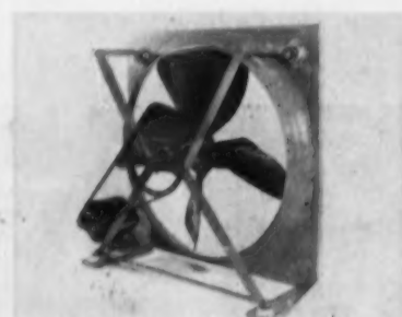
AB15283—ATTIC FAN —McLean Engineering Laboratories, Dept. AB, Box 531, Princeton, N. J. The firm's new line of low-cost attic fans have flexible frame for vibration absorption, neoprene shock mounting to reduce sound, may be used for horizontal or vertical discharge. No rubber or springs required. Each fan test-run before shipping to pre-set belt tension and pulley alignment. 20, 24, and 30 in. sizes.
