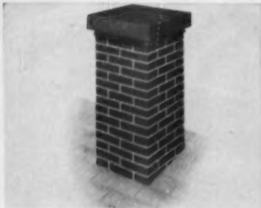
AB15152—PACKAGED CHIMNEY—SHERMAN, BOOTH 599 —General Products Co., Dept. AB, Fredericksburg, Va. This is a new chimney unit with an authentic brick-look chimney top. Trade name is Air-Jet Brick Beauty. The design is of embossed aluminum, construction finished brick red with depressed off-white mortar lines. The chimney weighs about 100 pounds, is UL approved for use with oil, coal, wood or gas fuels.
