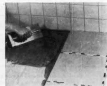
AB15178 — CLAY TILE MASTIC — SHERMAN, BOOTH NO. 485 —Minnesota Mining & Mfg. Co., Dept. AB, 423 Piquette Ave., Detroit 2, Mich. Faster, lower-cost installation of clay tile with new synthetic rubber adhesive is claimed by maker. Called CTA-11, adhesive is ready for use as taken from can. One pound of adhesive is said to do the work of 40 pounds of mortar. Coverage is 60-70 sq. ft. per gallon using the notched trowel specified.
