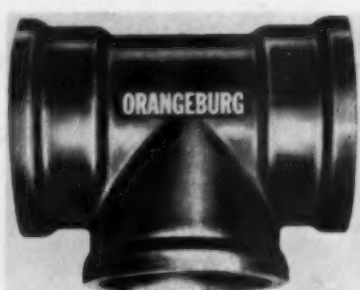
AB15293 — TEE FITTING — Orangeburg Mfg. Co., Inc., Dept. AB, 488 Madison Ave., New York 22, N. Y. The Tee shown here is made in 3-in. and 4-in. sizes and a new 3 1/4-in. bend is also in production. This non-metallic pipe and fittings is light in weight, can be cut with a coarse-tooth saw and tooled in the field. Taperweld joints do not require caulking or compounds. Recommended for underground non-pressure uses.
