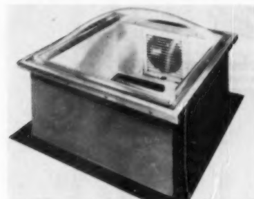
AB15080 — VENTDOME—HILTON, BOOTH 376 —Wasco Flashing Co., Dept. AB, Cambridge, Mass. Bringing daylight and ventilation to an interior room, unit consists of a white translucent or colorless plastic dome atop an extruded aluminum frame, and one or more motor-operated built-in air exhausts. Secured to roof deck by means of an extended roof flange, the "Ventdome" is particularly suited for inside baths.
