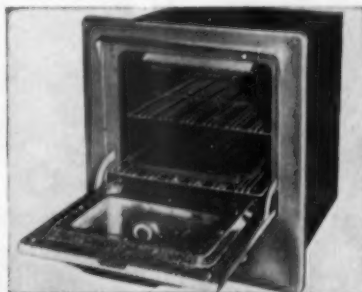
AB15120—WALL OVEN—HILTON, BOOTH 379 —Criswold Mfg. Co., Dept. AB, Erie, Pa. "Aristocraft" oven is completely self contained and ready to install, requires no additional insulation or exterior vents. Front trim of fully automatic unit measures 23 \times 26\frac{1}{2} inches; interior is 16 \times 15 \times 19 inches. Exterior finish is stainless "lifetime" satin chrome. Electrical rating: 118/236 volts AC, 3-wire single phase 60 cycle service.
