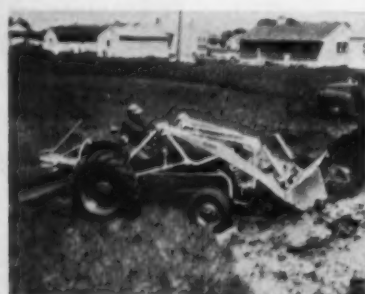
AB15291—WHEEL TRACTOR —The Oliver Corporation, Dept. AB, Merchandising Dept., 400 W. Madison St., Chicago 6, Ill. A new all-purpose wheel tractor known as the Super 55, designed for both industrial and farm service. It is suited for work with all types of attachments and has a built-in hydraulic system with finger-tip control for a 3-point hitch. Also double disc brakes.
