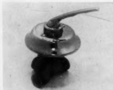
AB15059—SHOWER VALVE—SHER- MAN, BOOTH 553—Moen Valve Co., Div. of Ravenna Metal Products, Dept. AB, 6518 Ravenna Ave., Seattle 5, Wash. Model 20B controls temperature and volume with single handle and valve. Unit has no bib washers. User can pre-select water tempera- ture; change volume, turn it on and off, without affecting temperature. Available single, in tub and shower sets with semi- automatic or manual diverters.
