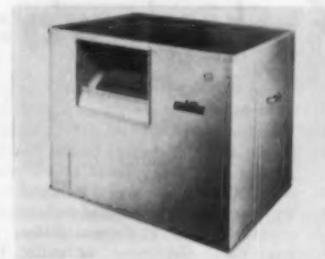
AB15201 — COOLING UNIT FOR WARM AIR SYSTEM — HILTON, BOOTH 377 —United States Air Conditioning Corp., Dept. AB, Como Ave. Southeast at 33rd. Minneapolis 14, Minn. This Kooler-aire air-cooled condensing unit can be used to convert a warm air heating system to all-year air conditioning. It is combined with a direct expansion coil installed at any point in the air supply system. Two models—2-ton and 3-ton.
