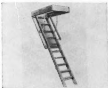
AB15058 — FOLDING STAIRWAY — SHERMAN, BOOTH 524 —Precision Parts Corp., Dept. AB, 400 N. First St., Nashville, Tenn. Simplex "balanced action" folding stairway has No. 1 kiln-dried lumber, heavy galvanized steel hardware, steps morticed into runners, all parts secured by bolts and screws. Fits 26x54-inch ceiling opening and comes in two sizes—8'3" and 9'9". Parts are interchangeable. Shipped completely assembled.
