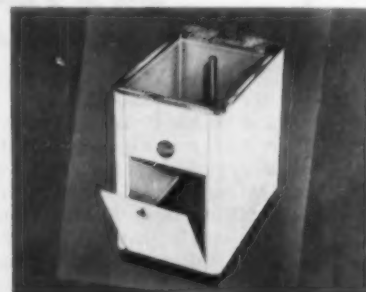
AB15082—LAUNDRY TUB — SHERMAN, BOOTH 403 —Wessels Co., Dept. AB, 1625 E. Euclid Ave., Detroit 11, Mich. Styled to match modern automatic washers and dryers, this compact unit measures 35\frac{1}{2} x29x19 \frac{1}{4} inch over-all. Twenty-one gallon capacity Fiberglas tub is said to do the job of 2-part tub merely by inserting overflow tube. Washing supplies can be kept handy in 19x29x16-inch storage area below tub.
