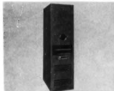
AB15064 — DOWN-FLOW CONDENSER—SHERMAN, BOOTHS 427-428 —Janitrol Heating & Air Conditioning Div., Surface Combustion Corp., Dept. AB, Columbus, Ohio. Designed for perimeter heating in slab or crawl space homes, gas-fired unit sizes are 80-100-120,000 Btu input. Blower sized to operate with conventional or small duct systems. Unit has exclusive Janitrol Multi-thermex heat exchangers, ribbon flame burners.
