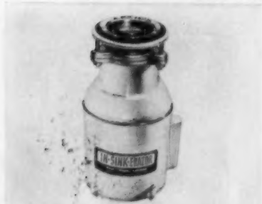
AB15342—FOOD WASTE DISPOSER —In-Sink-Erator Manufacturing Co., Dept. AB, Racine, Wis. This food waste disposer features automatic reversing action; continuous feeding and simple self-service all coupled with a new, silent operation. Installation is simple: cover flange is set in sink drain opening and a snap ring locks it in place. A slotted hook-on flange on disposer makes a simple, fast "hook" to cover flange; no special device needed.
