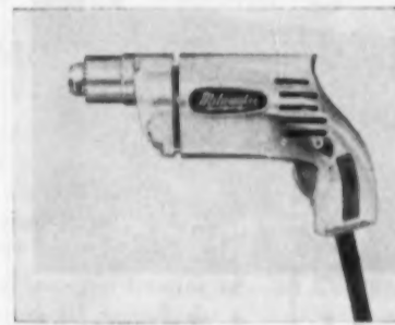
AB15284 — HEAVY-DUTY DRILL —Milwaukee Electric Tool Corp., Dept. AB, 5316 W. State St., Milwaukee 8, Wis. The new Series B, 1/4-in. electric hand drill is a 2.8 ampere, 115 volt, AC-DC universal motor with compound reduction gearing, has functionally styled grip that fits snugly into palm of hand. Weight is 3 1/2 lbs. Available in 6 models of chuck capacities of 1/2, 5/16 or 3/8 in. Price for 1/4-in. models: $42.00.
