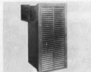
AB15072—RECESSED WALL HEATER—HILTON, BOOTH 39 —U. S. Machine Div., Stewart-Warner Corp., Dept. AB, Lebanon, Ind. Especially designed for closet or alcove installation, center vented, automatic heater adapts to prefabricated chimney, has optional snap-in outlet grilles for slides and rear. Oil-fired unit output is 60,000 Btu; gas-fired model input ranges from 64,000 to 75,000. Manual switch operates 10-inch fan in summer.
