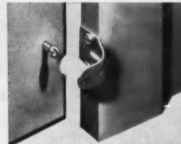
AB15171 — FRICTION CATCH — SHERMAN, BOOTH 419 —Washington Steel Products, Inc., Dept. AB, 1940 E. 11th St., Tacoma 2, Wash. This modification of this company's "1125" friction catch, for stile rather than shelf mounting, incorporates the catch on a curved steel mounting base, allowing installation for lipped doors. Known as "Washington 1126," the new catch is of a material unharmed by acids, moisture or temperature changes.
