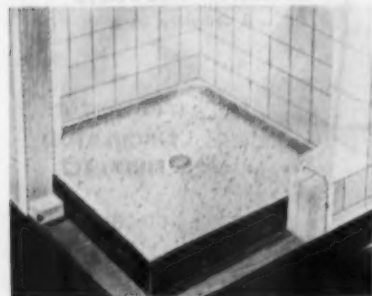
AB15350 — SHOWER RECEPTOR — SHERMAN, BOOTH 475 —Fiat Metal Mfg. Co., Dept. AB, 9301 W. Belmont Ave., Franklin Park, Ill. Said to replace two trades in its installation compared to built-up shower floor, precast receptor has monolithic construction that eliminates leakage. Made in either artstone or terrazzo for showers with walls of tile or plaster, receptor has drain, removable strainers, tiling-in flange.
