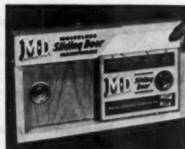
AB15275—FASCIA STRIP —Macklanburg-Duncan Co., Dept. AB, Box 1197, Oklahoma City, Okla. An optional item in sliding door hardware line, new FM-300 fascia strip is made of extruded aluminum with a silvery-satin finish. As illustrated in the operating model above, strip is attached directly in front of overhead track, covers all exposed hardware, eliminates further need for wood trim. Comes in standard lengths for any opening.
