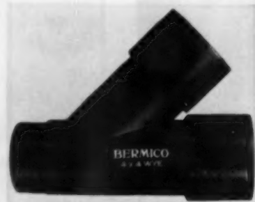
AB15379—SEWER PIPE —Brown Co., Dept. AB, 150 Causeway St., Boston 14, Mass. This Bermica root-proof sewer pipe is chemically resistant to ground acids and ground alkalis; withstands freezing and thawing, and will not tuberculate, corrode or disintegrate in service. It is manufactured in 8 foot lengths of 2, 3, 4, 5 and 6 inch inside diameter. Fittings are Tee, Wye, 1/4 Bend, 1/2 Bend. Easily assembled; no pipe compounds needed.
