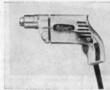
AB15284 — HEAVY-DUTY DRILL —Milwaukee Electric Tool Corp., Dept. AB, 5316 W. State St., Milwaukee 8, Wisc. The new Series B, 1/4-in. electric hand drill is a 2.8 ampere, 115 volt, AC-DC universal motor with compound reduction gearing, has functionally styled grip that fits snugly into palm of hand. Weight is 3 1/2 lbs. Available in 6 models of chuck capacities of 1/2, 5/16 or 3/8 in. Price for 1/4-in. models: $42.00.
