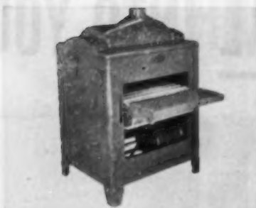
AB15331—24-INCH SINGLE DRUM SANDER —Woodworkers' Tool Work, Inc., Dept. AB, 222 So. Jefferson St., Chicago 6, Ill. This non-oscillating 24-in. Drum Endless Bed Sander is 24 in. long 14 in. diameter, felt covered, spring-action lock keeps sandpaper tight. Has rate of feed 15 to 30 feet per min. Takes material to 6 in. thick or short pieces 16 in. long. 3 Hp motor, 220 Volt 3 Ph. or 110/220 Volt, Single Ph.
