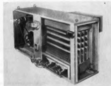
AB15098—HORIZONTAL FURNACE—SHERMAN, BOOTHS 579-580 —Armstrong Furnace Co., Dept. AB, 851 W. Third Ave., Columbus 8, O. Ideally suited for attic, crawl space and a wide range of suspended installations, compact gas-fired horizontal unit is made in 70,000, 85,000, 105,000 and 135,000 Btu sizes; largest measures only 51 in. long, 21 1/2 in. deep, 24 in. high. Furnace also features filter rack built into blower compartment.
