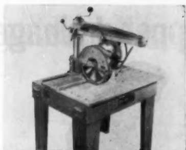
AB15381 — RADIAL ARM MULTI-PURPOSE MACHINE — HILTON, BOOTH 157; SHERMAN, BOOTH 586 —DeWalt Inc., Dept. AB, Lancaster, Pa. Called GWI, DeWalt's latest machine is equipped with a motor that will develop 1½ h.p. and is provided with voltage-change switch for use with 115 or 230 volt, single phase current. With 10-in. blade (standard) unit's cutoff capacity of 1-in. material is 16 in. Maximum depth of cut is 3 in.
