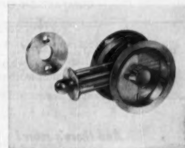
AB15225 — SLIDING DOOR LOCK —Adams-Rite Mfg. Co., Dept. AB, 540 W. Chevy Chase Drive, Glendale 4, Cal. Known as Series 660, this lock operates with a smooth snubbing latch action due to the simple ball-shaped bolt. The lock is reversible on the job and fits any door from 1 3/4 in. to 1 3/8 in. Locking and non-locking escutcheons can be interchanged. Thumb button provides positive security.
