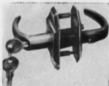
AB15290 — SCREEN AND STORM DOOR LOCK —National Hardware Co., Dept. AB, Ozone Park, N. Y. One-piece assembly simplifies installation of this new solid aluminum screen and combination storm door cylinder key lock. It is adjustable for metal and wood doors 3/4-in. to 1 1/2-in. thick. Has push-button action with inside locking device. Lockset can be locked and unlocked freely from inside and out at all times.
