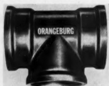
AB15293 — TEE FITTING —Orangeburg Mfg. Co., Inc., Dept. AB, 488 Madison Ave., New York 22, N. Y. The Tee shown here is made in 3-in. and 4-in. sizes and a new 3 1/2-in. bend is also in production. This non-metallic pipe and fittings is light in weight, can be cut with a coarse-tooth saw and tooled in the field. Taperweld joints do not require caulking or compounds. Recommended for underground non-pressure uses.
