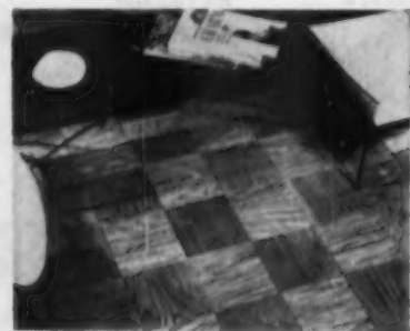
AB15388—OAK BLOCK FLOORING —SHERMAN, BOOTH 473 —Wood-Mosaic Co., Parkay Div., Louisville, Ky. This new, prefinished laminated block flooring features one-piece face of oak and waterproof plywood construction. Blocks are 9x9-inch squares, 3/8 in. thick, t&g with slightly beveled edges. Faces are factory-finished, waxed and polished. Application is with adhesive over any smooth subsurface—slabs on grade, plywood or wood.
