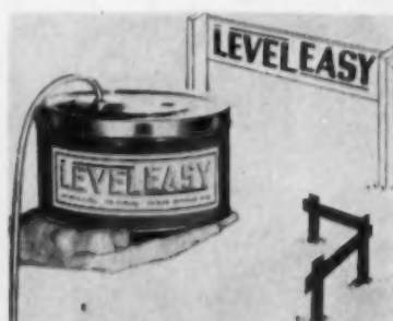
AB15256—WATER LEVEL —Hydro-level, Dept. AB, 53 DeSoto, Ocean Springs, Miss. "Leveleasy" is a simple water level, hand size, made up of a fluid reservoir, tube reel and 50-ft. clear plastic tube permitting extension of level line for 100 ft. A mechanic's tool, one man can use it for setting batters, grade stakes, setting tile, concrete floors, in masonry work, form erection or setting screeds. Price $7.95.
