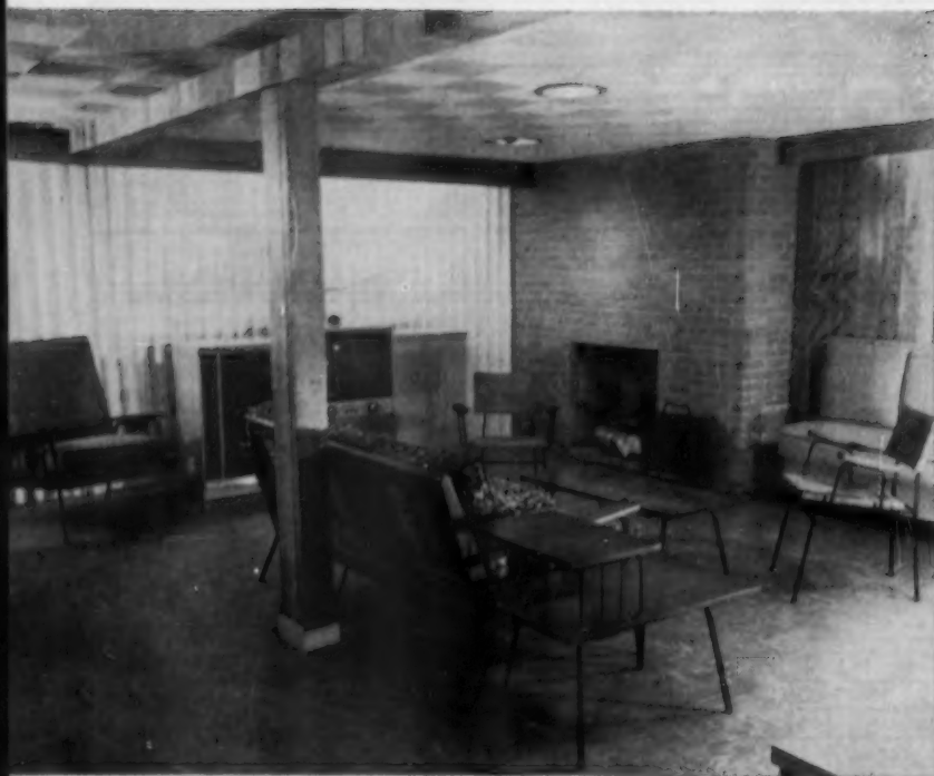
Dimmer-control for cornice lighting over corrugated curtain wall gives changing intensity of colored light. Note that the birch cornice board and mounting board for the fluorescent tubes are angled
