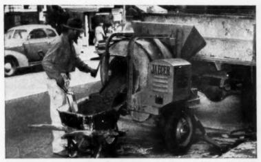
Same wages . . . 12 to 15 yards more concrete: Fastest half-bag mixer built —the  $3\frac{1}{2}$ S Auto-Loader. You load while you mix, then charge in a flash with automatic shaker hopper. Has equally fast discharging action and same rugged construction as Jaeger 6S, 11S and 16S power loaders. Ask for Catalog.
