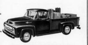
**MAX. GVW: 5000 LBS.** 8-foot (65.4 cu. ft.) body on 118inch wheelbase gives biggest loadspace of any halftonner. Even Standard  $6\frac{1}{2}$ -foot body on a 110-inch wheelbase has more capacity than most other pickups. Tubeless tires on *every* model, at no extra cost.
