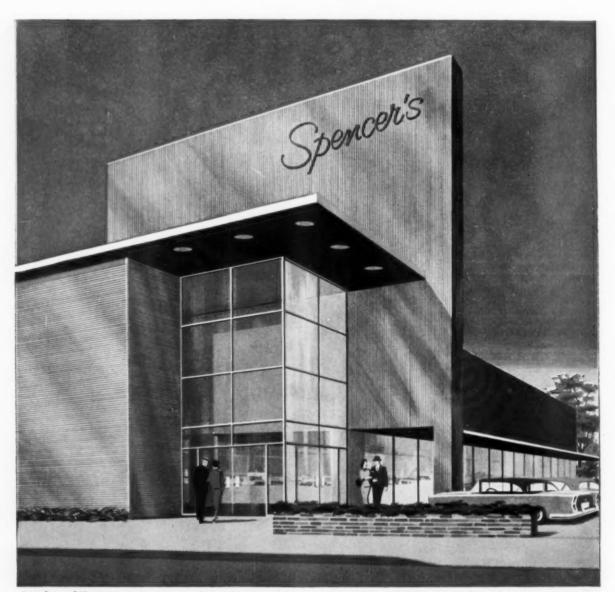
Facades and Marquees made with strong Kaiser Aluminum have an ideal variety of texture finishes . . . may be painted, anodized, embossed, enameled, lacquered, and porcelainized by standard methods. They weather uniformly, never rust, never stain-require minimum maintenance. Lightness lowers erection costs. Available in flat, corrugated or specially designed panels. Their application provides a distinctive quality to any building... and helps assure client satisfaction.
