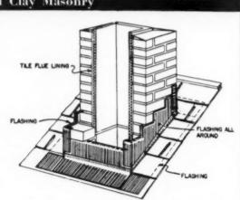
Base flashing of chimneys should extend well back under the roof covering. Counter flashing should be imbedded securely in the mortar joints of the chimney wall. .
