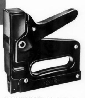
**BOSTITCH T5-8 TACKER** is the handiest fastening tool a builder can own. Gets into tight places. Drives  $\frac{1}{4}$ " staples for screening,  $\frac{3}{8}$ " staples for fastening insulation,  $\frac{1}{2}$ " or 9/16" staples for flanged ceiling tile.
