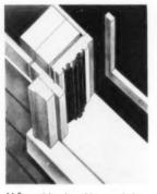
$\frac{1}{2}$ " outside sheathing and drywall ( $\frac{3}{6}$ " or  $\frac{1}{2}$ ") inside on 2 x 4's, cut-off rib on blind stop and remove inside jamb strip.
