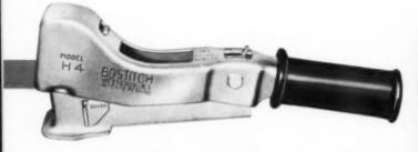
**BOSTITCH H4 HAMMER** drives a rugged  $\frac{3}{4}$ " galvanized staple which spreads inside the wood for an anchor grip. Thus *one* blow with *one* hand drives the equivalent of *two*  $\frac{3}{4}$ " nails of  $\frac{1}{16}$ " wire.
