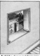
**Build the sleeve** and frame into wall during construction. Opening is about 23" high by 27" wide. This is easy to do in modernizing present homes, too.
