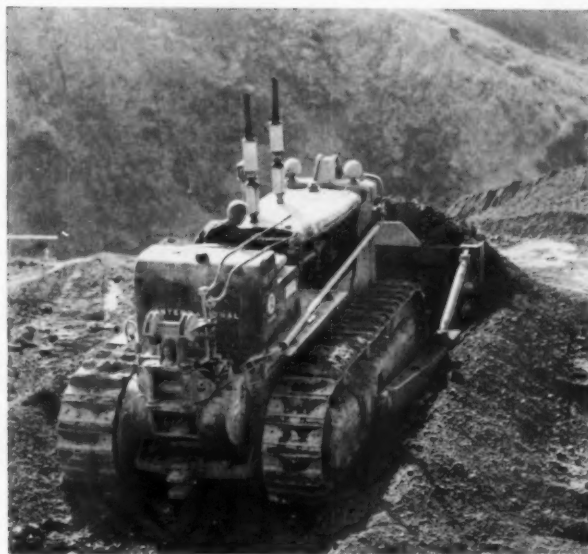
JACK OF ALL TRADES is the big bulldozer. It can cut, push dirt, and tow other pieces of heavy equipment.
