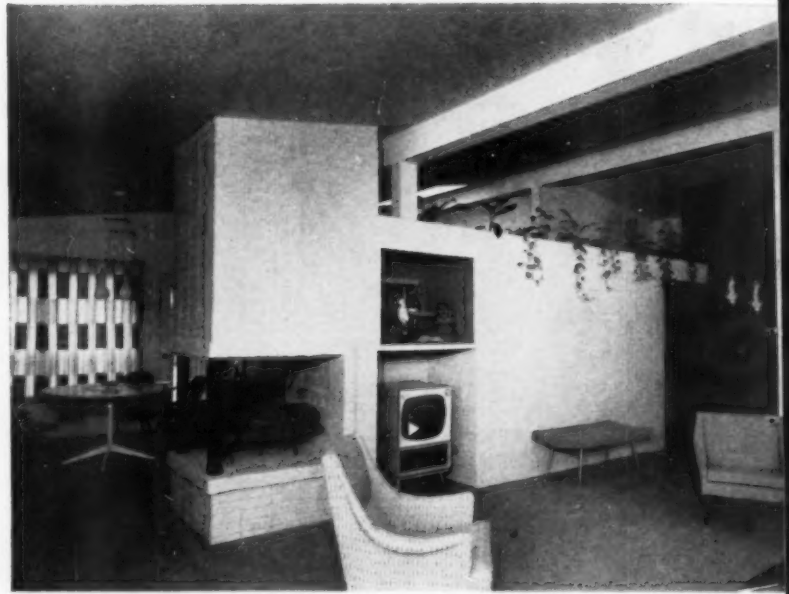
A ONE-ROOM REVIEW of current trends: two-way fireplace with corner columns; set-in TV; high-level planter; roman brick divider; exposed beam; glamor lighting; skylight. Andrews-Wood, Birmingham .
