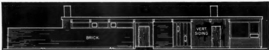
FRONT or north elevation shows extended bedroom wall (1) and child's room (right).
