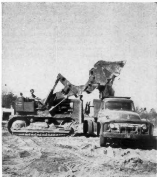
COMBINATION BULLCLAM AND SKID SHOVEL can push dirt, load it as shown, or transport it. International-Harvester Tractor. (Circle 12060, p. 142.) "Four-in-one" shovel, Drott Mfg. Co. (Circle 12060A, p. 142.)
