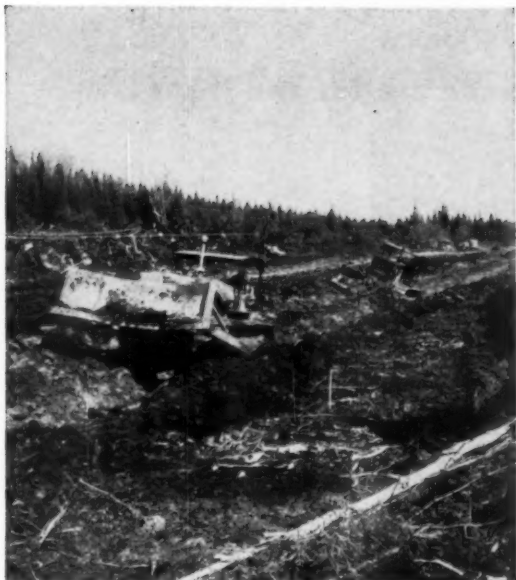
THE "U" BLADE has its sides advanced ahead of its center, can push a bigger load with less side spill. Pointed corners help penetrate hard soil, dig under rocks. Caterpillar Tractor Co., Peoria, Ill. (Circle 12058, p. 142.)
