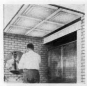
MODULAR LIGHTING in panels of 2'x2' or in complete Sunshine Ceiling package for standard 5'x7' and 5'x8' bathrooms. Ceilings "float," do not touch walls, allow ample air circulation. Electrical channels attach to structural ceiling with grid to hold diffusers. Wakefield Co., Dept. AB, Vermilion, Ohio. (No. 5003, p. 132.)
