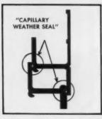
Bourne Capillary Seal keeps out rain, wind, and dust around all vent openings.
