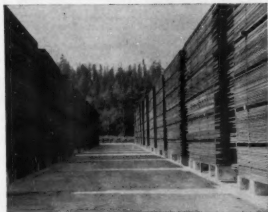
Each unitized stack is made up of lumber in classifications according to green weight, and remains in the yard until moisture content reaches a specified range.
