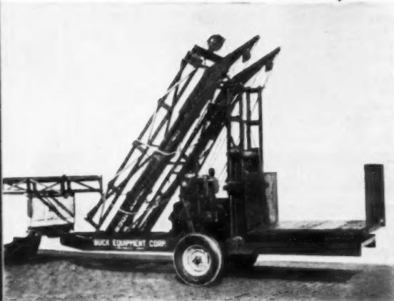
**TO ERECT HOIST:** turn on motor, throw out clutch. Hoistower is self-erecting and rises as wheels retract to its 45' unloading height.
