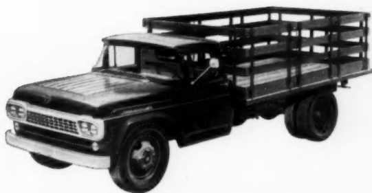
New Ford F-500. Rugged, versatile 1½-tonner with 15,000-lb. GVW. Two wheelbases for 7½- to 13-foot bodies.
