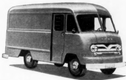
New Ford Parcel Delivery chassis. Four P-Series chassis with GVW's from 8,000 to 17,000 lb., for up to 525-cu. ft. custom bodies.
