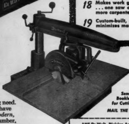
MODEL MB-F WITH 9" SAW. Portable, with new ¾ hp direct-drive motor, 120 V. 9" all-purpose saw blade cuts 2½" deep, rips 24" wide, cross-cuts 15" wide on 1" stock. Safety key switch, safety guard, and anti-kickback device. Weighs only 140 lbs.
