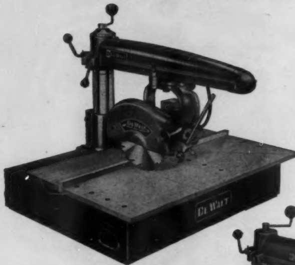
MODEL 6W-1 WITH 10" SAW. With 1½ hp direct-drive motor, 120/240 voltage change switch. 10" saw blade cuts 3" deep, rips 26" wide, cross-cuts 18" wide on 1" stock. Steel base with welded carrying handles, carries through 30" door. Safety key switch, guard, anti-kickback device. Weighs only 183 lbs.
