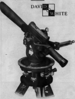
For Concrete Contractors—You will enjoy using this versatile, low-cost instrument. Determine differences in elevation, run lines for curbs, plumb walls, lay out angles. Rugged construction. New, streamlined styling. T8007 Light Construction Level-Transit—Tripod included. Retails for \$89.50.
