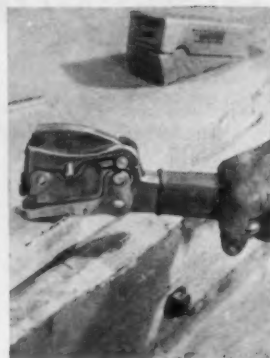
ONE BLOW of hand stapler places and drives staple home, freeing other hand to position work. Tool above is in wide use installing tile, insulation.
