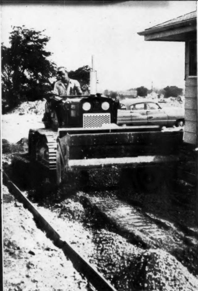
Clam-action International Drott 4-in-1 combines standard bucket, bulldozer, carry-scraper, and clamshell in one machine.
