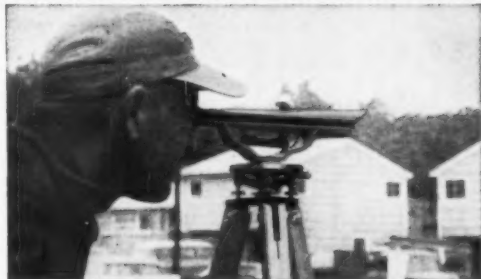
SPEED-A-LINER DUMPY LEVEL — Model 190 — 18-power internal focusing 11½" telescope. Understung level vial fully protected. Built-in sunshade. Enclosed 4-screw leveling head. $69.95*
