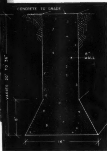
DITCHER RIG DIGS —Combination rig simultaneously digs trench 3 ft. deep and carves bell-shaped footing into fill.
