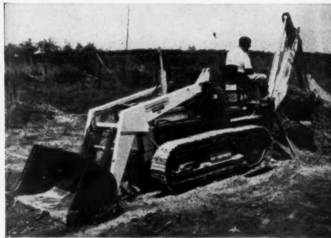
Dig 10 feet deep with rugged International Wagner backhoe; backfill, load with sturdy 3,500 lb capacity loader.
