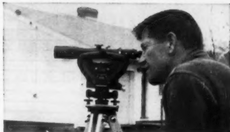
MASTER BUILDER CONVERTIBLE TRANSIT-LEVEL — Model 320 — Big instrument performance at moderate cost. 22-power telescope; coated optics, 3-ft. short focus. Powerful leveling lock. $229.50*
