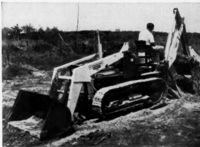
Dig 10 feet deep with rugged International Wagner backhoe; backfill, load with sturdy 3,500 lb capacity loader.
