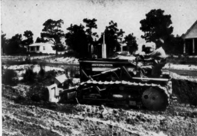
IH Bullgrader is raised, lowered, angled, and tilted hydraulically—all controlled from the tractor seat.
