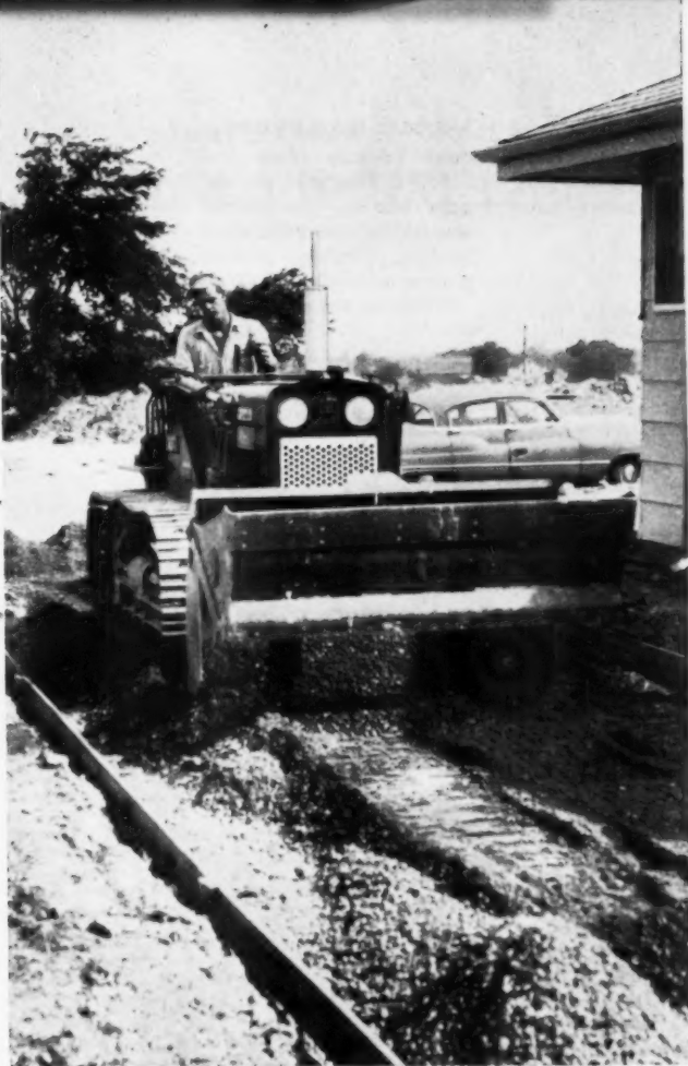
Clam-action International Drott 4-in-1 combines standard bucket, bulldozer, carry-scraper, and clamshell in one machine.
