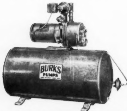
BURKS MULTI-STAGE CENTRIFUGAL. Greater capacities at higher pressures from deeper settings. Compression type fittings. Two- and three-stage pumps—1/2 through 1 1/2 hp sizes with capacities to 2310 gph. All bronze pumping parts. Pump installs horizontally or vertically.
