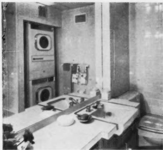
STACKED WASHER-DRYER in bathroom is sales feature. So are large mirrors, which reflect smaller bathrooms into large ones. High-pressure laminate countertops in contrasting colors accent colored fixtures, tile; care is easy.
