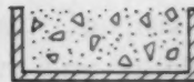
COARSE AGGREGATE LESS TOTAL SURFACE TO BE COATED WITH CEMENT — (MORE ECONOMICAL)
