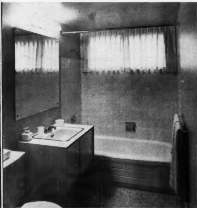
WALL-HUNG LAVATORY , in bathroom, is built into decorative cabinet with sliding plastic doors beneath. Centrally located bath is convenient to bedrooms, adjacent to linen closet.
