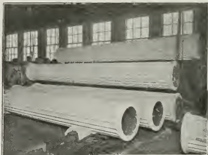
Concrete Columns of a Large Type in the Factory
