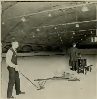
The Electrically Drawn Ice Planer Preparing the Ice Surface for Skating
