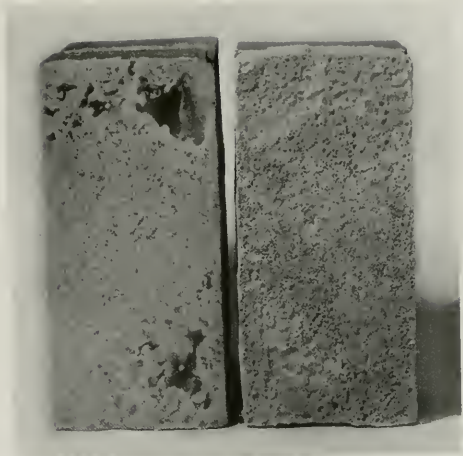
Figure 2—Same bricks and mortar as illustrated in Figure 1. In this case, bricks were 50 per cent saturated when laid. Note underbonded areas on brick surface.
