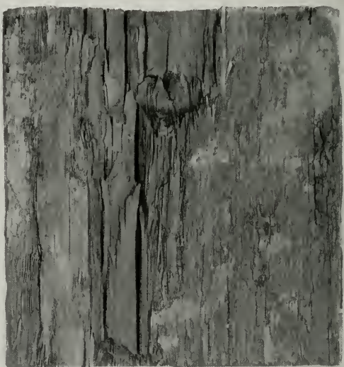
FIG. 6—SPECIMEN CONTAINING LESS THAN ABOUT 11½ PER CENT OF HOT-WATER-SOLUBLE EXTRACTIVE DO NOT RESIST ATTACK BY FUNGI
