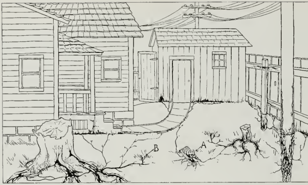
Fig. 28—This sketch combines the sorts of conditions found to prevail in many localities where wood has been improperly used. Unprotected wood in or on the ground makes possible both settlement and rapid increase of the subterranean termites. Workings in stumps, poles, posts, sidewalks, and wood of buildings are shown in black, as are the galleries within the earth. A marks the supposed original point of entry of one of the colonizing pairs, and B the points of emergence of swarming alates at the proper season.
