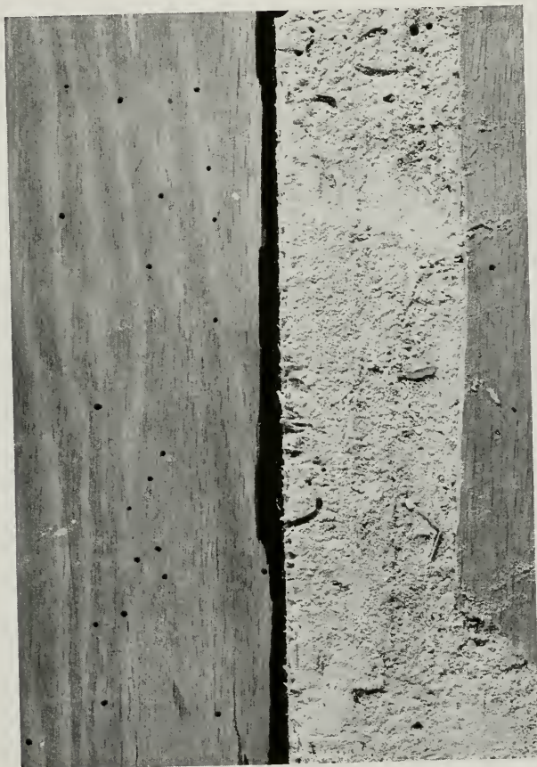
Fig. 5—Work of a typical powder-post beetle, fig. 1-b, in oak flooring. Left, surface showing adult emergence holes. Right, work of larvae exposed by removing surface layer. When these typical "shot" holes appear on the surface of any article made of oak, ash, hickory, or mahogany, it would be well to investigate.
