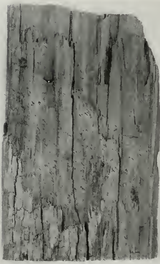
FIG. 6—SPECIMEN CONTAINING LESS THAN ABOUT 11½ PER CENT OF HOT-WATER-SOLUBLE EXTRACTIVE DO NOT RESIST ATTACK BY FUNGI
