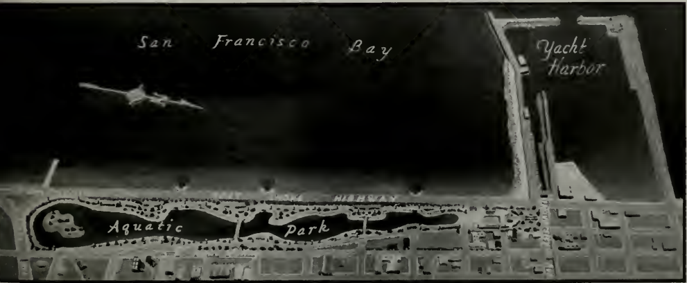
PLAN FOR DEVELOPMENT OF WATERFRONT, BERKELEY, CALIFORNIA With Federal aid Berkeley's waterfront is being transformed from muddy tidelands into a beautiful aquatic park and yacht harbor. The Eastshore Highway, which will be Berkeley's major arterial to the San Francisco Bay Bridge, will provide a natural tidal basin for the development of an aquatic park. Total cost of the project is estimated at $1,000,000.
