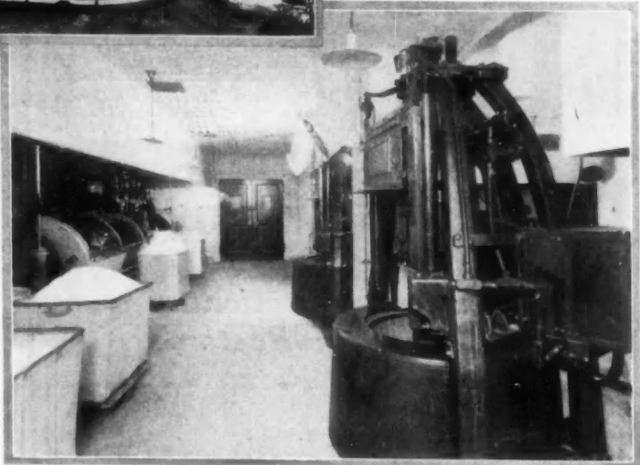
A section of the washroom—equipped with Cascade washers and Humatic extractors.
