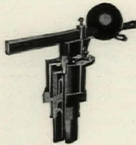
Cut open view of No. 45-A Sylphon Hot Water Damper Regulator. Controls from 120 deg. to 220 deg. F. Length of bulb 2 inches; threaded 2-inch pipe size. Installed in a Y or screwed into boiler.
