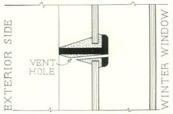
Full size section showing method of venting air space through steel sash by boring holes in muntin bars, necessary where windows are fixed.
