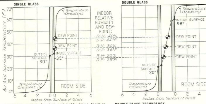
Temperature gradients for single and double glazing, based on tests by A.S.H.V.E. Research Laboratory. Curves show that double glass raises inside surface temperature to 58° F., well above room dewpoint, thus preventing condensation.
