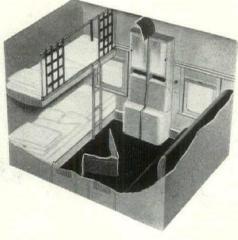
Six types of rooms are provided on the Pullmans used by the new Pennsylvania and New York Central trains. Two of these are shown above. The double bedroom contains a lavatory and watercloset; a number of these units are separated by folding partitions so that additional space can be obtained if desired. The Roomette is a private room with one bed and complete toilet facilities.
