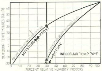
Curves showing point at which condensation will occur, single and double glass windows, for various outdoor temperatures and indoor relative humidities.
