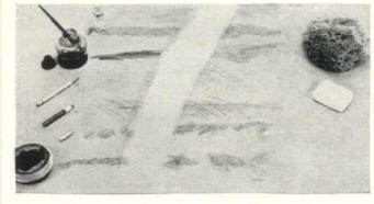
This test panel is a 2' x 3' piece of wallboard, painted with Dutch Boy White-Lead and Lead Mixing Oil. For a solid week, this panel lay in a busy corridor. It was walked on by hundreds of people daily. Horizontal streaks show how it was then defaced with grease, ink, pencil, crayon, shoe blacking, lipstick, etc. Swath shows marks completely removed by washing with soap and water.
