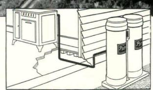
This diagram illustrates the basic simplicity of the "PYROFAX" Gas installation. Two types of equipment are provided. In Type "T," as shown in sketch above, the cylinders are not enclosed in cabinet. Type "A" Cabinet equipment completely encloses the cylinders.
