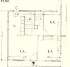
TYPE D covers three buildings of three units each. One unit is shown above. The plan is somewhat more conventional than the others shown. Good use is made of the offset units to gain more light and air.
