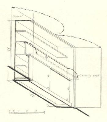
The simplest type of residential bar is that which occupies a large closet, as in the example above. Double doors open the full width of the recess, and a folding counter provides a work shelf for mixing drinks. The outdoor recreation room shown below is enclosed on one side by a glazed wall to keep out the weather, spans the space between the garage and the house. A two-way bar opens both into the porch and a smaller, inside den.
