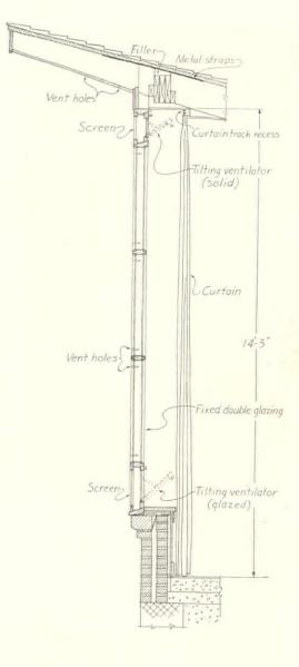
The fixed window, with small horizontal ventilator sash at top and bottom, has the advantage that no screens interfere with the view. Also, it is relatively easy to double glaze, thus avoiding large areas of cold glass. In the window above, ventilator panels are projected inward, with plenty of room between the window and the drape for the fully-opened sash.
