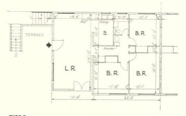
**TYPE E** shows an interesting apartment scheme, with an outside entrance to the upper floor and a terrace over the ground-floor living room. The construction is largely precast concrete, in the form of block and plank. As in the other schemes, kitchens are more or less open to the living rooms. Average cost per unit: \$2,641.
