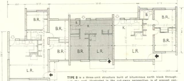
out; the roof, illustrated in the cut-away perspective, is of precast concrete units. The thick party walls, an integral part of the construction, offer a degree of soundproofing uncommon in houses of this price class. Average cost per unit: \$2,850.
