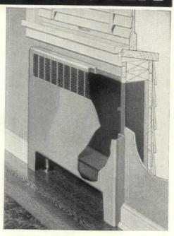
Projection Style Recessed Enclosure. Fronts may project 2½, 4½, or 6 inches forward of plaster line. Heating units up to 9¼ inches deep may be installed in 4-inch stud wall.
