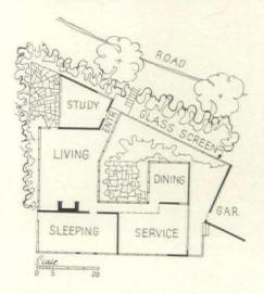
While exterior screens of transparent glass have been used occasionally, where a windbreak was required which did not shut off a view, the translucent wall used out of doors is not common. The main advantage would appear to be a decorative one, as plants can be effectively shown in silhouette against the bright background.
