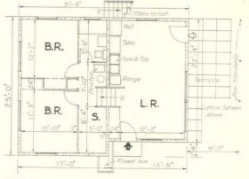
TYPE C is a single-family four-room house, built entirely of concrete. The plan divides into two approximately equal units, one slightly higher than the other. Cooking space is exposed. Cost: \$2,950.
