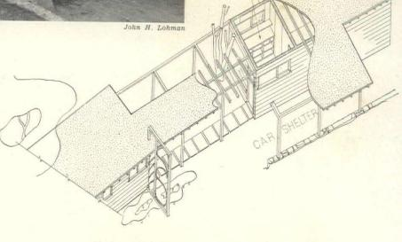
Above is an ingenious hook-up of garage, workshop, service entrance and laundry, connected by a shelter affording protected access in bad weather. The garage below, located at the front of the house, acts as a porte cochere and, since it is open at both ends, requires no backing and filling either going in or out.
