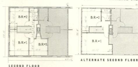
2 & 21/2 STORY UNITS. Based on the typical row house plan, this unit is designed with alternate top-floor plans which provide either two bedrooms per family or an additional bedroom spanning the party wall which may be attached to one or the other. A small, one-bedroom apartment is added on the low side of the ground floor on sloping sites.
