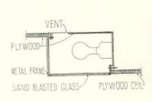
The living room shown here has a step-down ceiling, breaking up the space into high and low sections. As indicated by the drawing, a continuous lighting unit at the point where the break occurs is effective in accenting the change in levels, since it illuminates the high ceiling and leaves the lower one dark. Relamping is done by simply pushing up the loose panes in the soffit frame.
