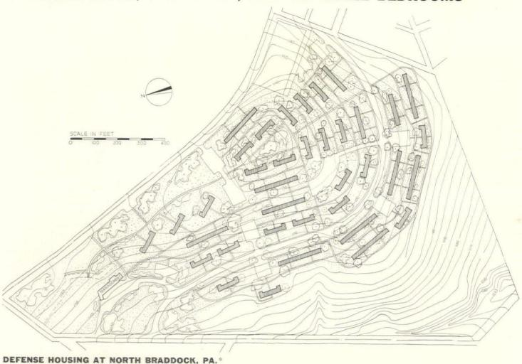
The row-type units of this 200-house project are arranged on the rounded end of a knoll, and face south, southwest, and west according to the direction of the slope. A single traffic street traverses the property in an easy curve, following the contours except at the ends, where it drops to the level of the adjoining roads. Parking areas at right angles to this street provide
