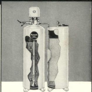
HOW IT WORKS—Water enters at top, flows through mineral bed, which extracts the hardness-forming calcium and magnesium, the softened water passing to service. When the mineral has removed its capacity of hardness, it is automatically regenerated by salt brine from the other tank. No salt taste gets into the water.
