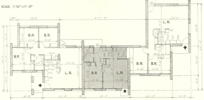
TYPE A provides the same accommodations as the unit above, and at the same cost, but uses cement-stabilized tamped earth walls instead of block. This structural method, a comparatively recent development, is reputed to have many advantages over the traditional rammed earth. Certain plan features are worth noting, especially the placing of the heater off the inside hall, and the use of fire-places partly to screen activities in the kitchen. Average cost per unit: \$2,850.
