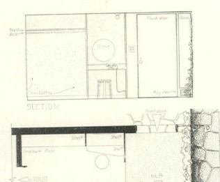
The space shown adjoins the entrance vestibule of a country house, and has a dressing and telephone table, and a rack for coats and hats. Where living habits are not too formal the openness of such a scheme should prove entirely acceptable. The perforations in the upper part of the screen wall allow the light in the closet to illuminate the vestibule.
