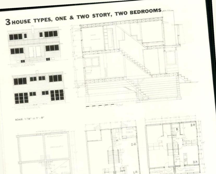
TYPE D (above) is a 2 story, single-family row house with 2 second-floor bedrooms and partial basement. Living, dining, and kitchen areas on the first floor are merged into one large space; a recessed, sheltered entrance has been added at the front, and a screened porch at the rear. The second floor plan is featured by a balcony running across the front and a small bunk room, opening off the larger of the two bedrooms and screened by prefabricated closet units.
