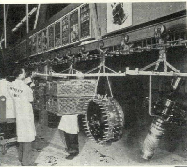
FIRST FLOOR OF MAINTENANCE SHOP IS DEVOTED LARGELY TO ENGINE OVERHAUL CONTINUOUS CHAIN CONVEYORS PROVIDE QUICK MOVEMENT OF EQUIPMENT, PARTS
