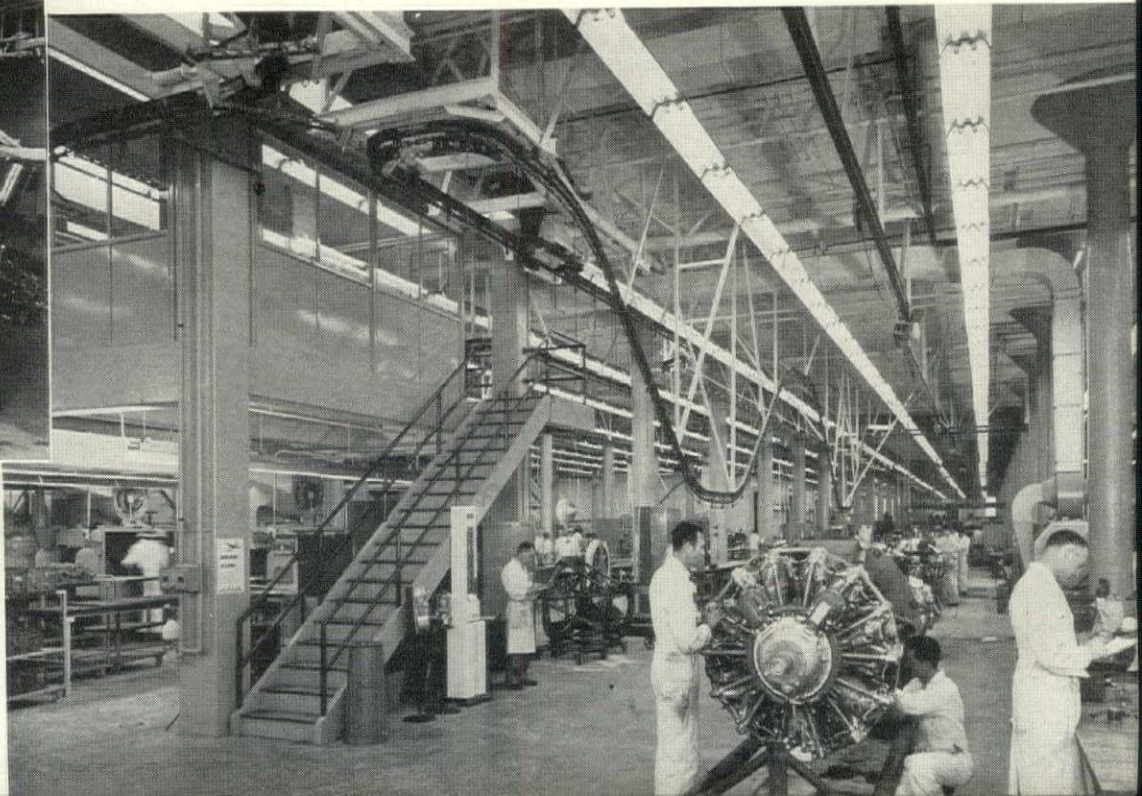
FIRST FLOOR OF MAINTENANCE SHOP IS DEVOTED LARGELY TO ENGINE OVERHAUL CONTINUOUS CHAIN CONVEYORS PROVIDE QUICK MOVEMENT OF EQUIPMENT, PARTS
