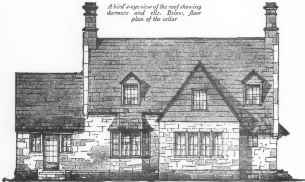
The rear façade of the American adaptation of the Cotswold house showing the quaint bay window at the end of the living room and the four casement windows in the dining room
